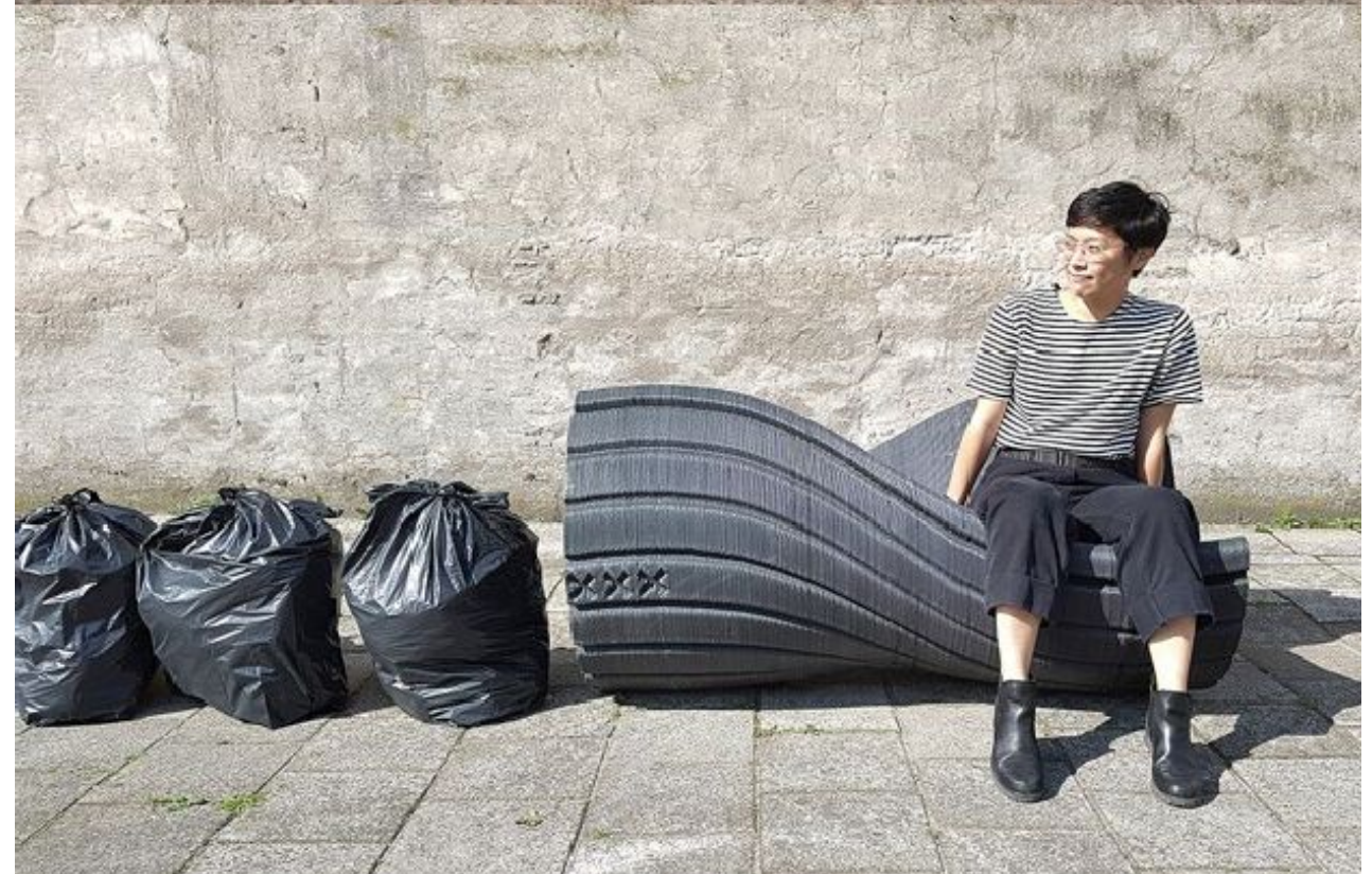
The new raw - Amsterdam // Zero Waste Lab - Thessaloniki 3D printed urban furniture using the city's trash
