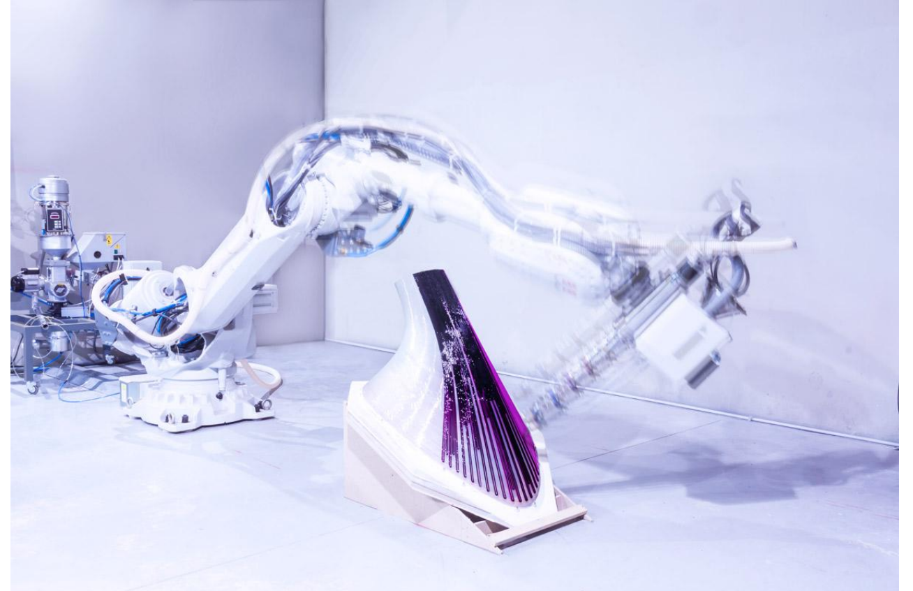
Nagami - design: Zaha Hadid, 3d printed chairs using pellets
